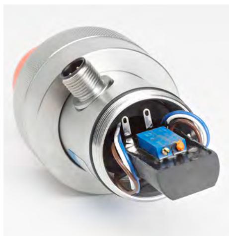
Internal View of Transmitter
